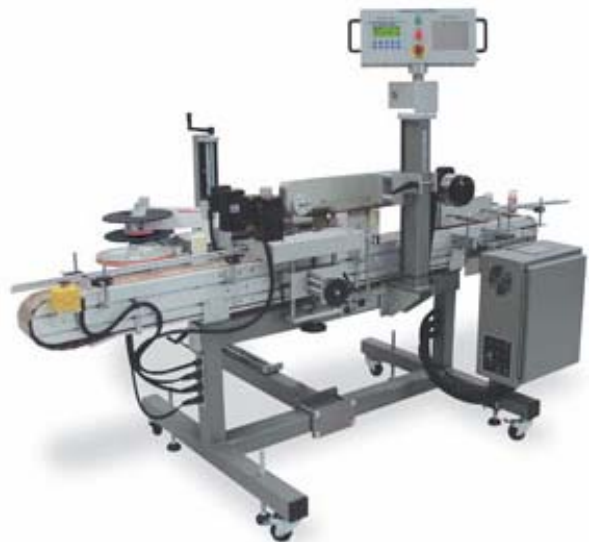
Open frame labeling system with spacer wheel and chain aligners configured to label both round- and oblong containers
